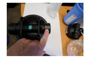
2. Mount the housing to the bracket using the supplied self-tapping screws, orienting the housing to match the applications desired flow direction. If you need to position the flow direction to right or left, the bracket will need to be turned 180 degrees.
